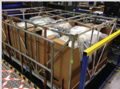
TUV vibration test – ISTA test standard on 6 engine corrugated dunnage
