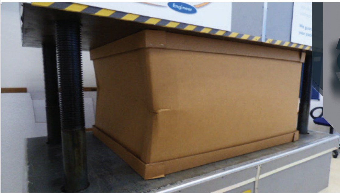
Compression test: test to failure at 3500kgs
