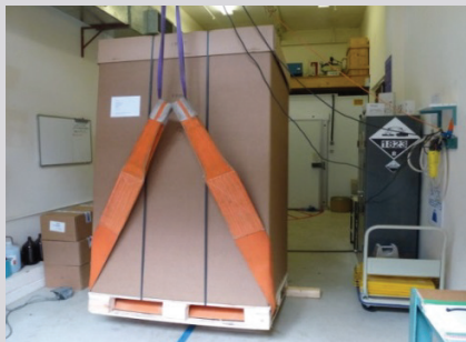
Drop Test- vertical tilt test on 500kg pack
