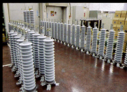
Polymer housed station class surge arresters
