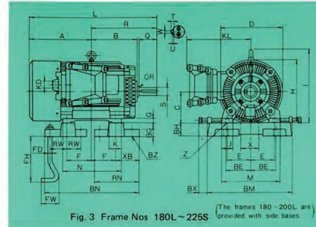
Fig. 3 Frame Nos 180L ~ 225S (The frames 180 ~ 200L are provided with side bases)
