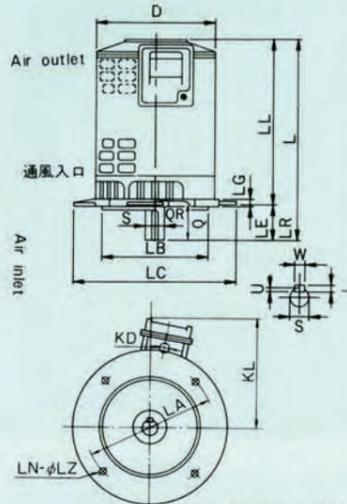
Fig. 1 Frame Nos 90L ~ 100L (Bracket tightening bolts for 6-pole and 8-pole machines are located outside the frame)
