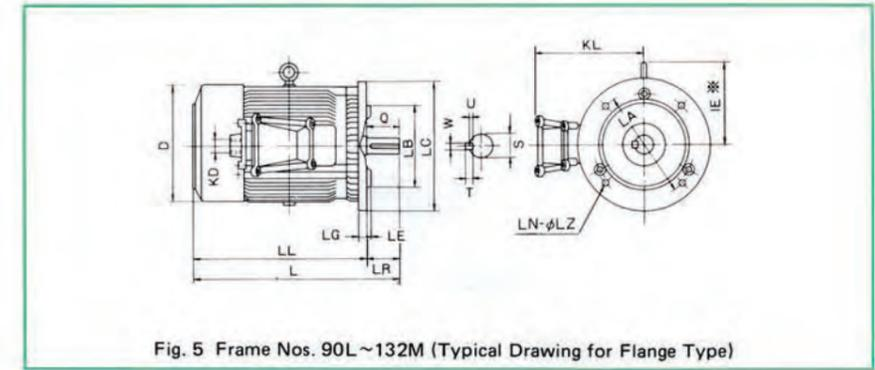
Fig. 5 Frame Nos. 90L~132M (Typical Drawing for Flange Type)
