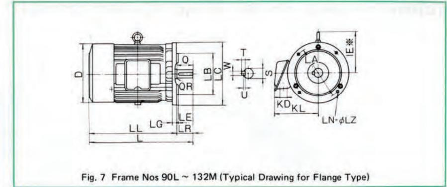
Fig. 7 Frame Nos 90L ~ 132M (Typical Drawing for Flange Type)
