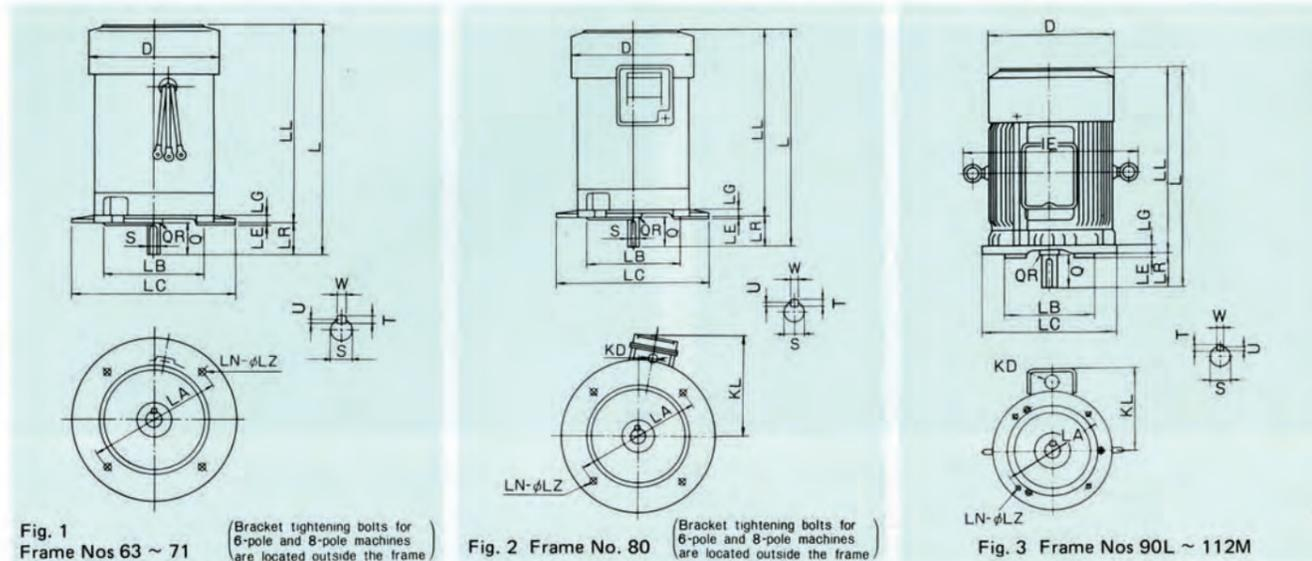
Fig. 1 Frame Nos 63 ~ 71 (Bracket tightening bolts for 6-pole and 8-pole machines are located outside the frame)
