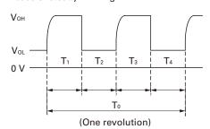
$T_{1 \text{ to } 4} \doteq (1/4) T_0$   $T_0 = 60/4N \text{ (s)}$   $N = \text{Fan speed (min}^{-1})$
