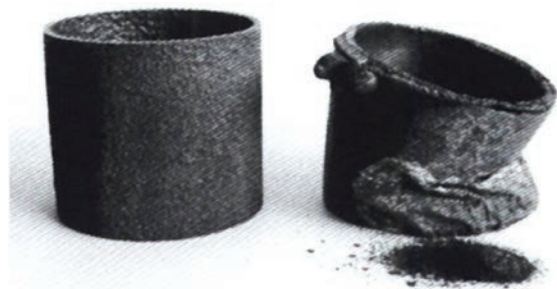
INEX @ 360 hours 600 Alloy @ 1 hour Si-SiC Composite vs. 600 Alloy (after just 1 hour) No deformation for the INEX tube 360 hours @2462
