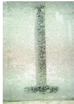
Disperion of Gas (Water model)
