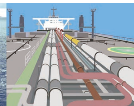
Cargo oil pipes
