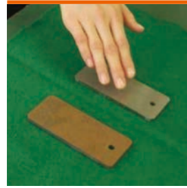
Red rust caused by contamination from human hands indoors
